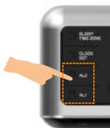
2. **Stop the alarm** : Press **AL1 / AL2** when the alarm is ringing.
